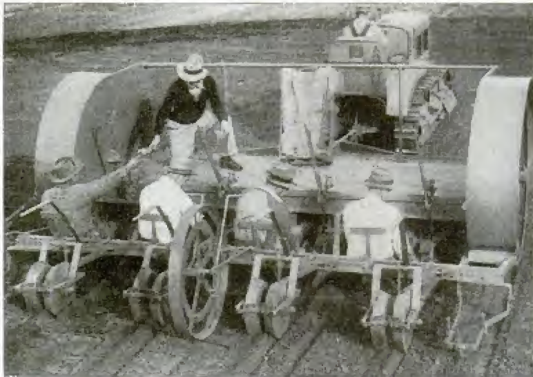
The four men seated at this machine can plant 240 guayule seedlings a minute. The machine prepares the hole and covers the new "rubber" plant
